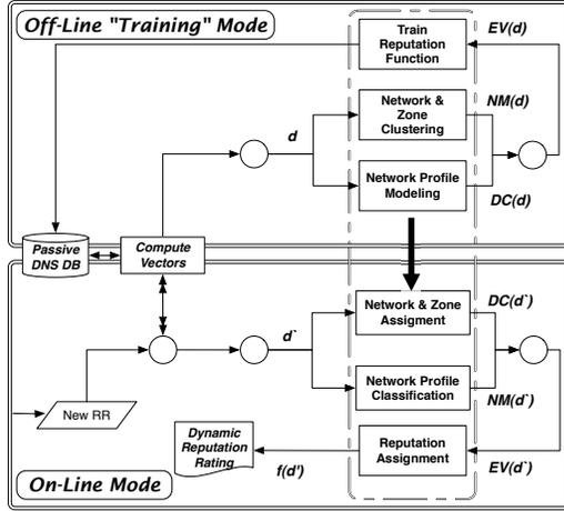
Figure 3. Off-line and on-line modes in Notos.
